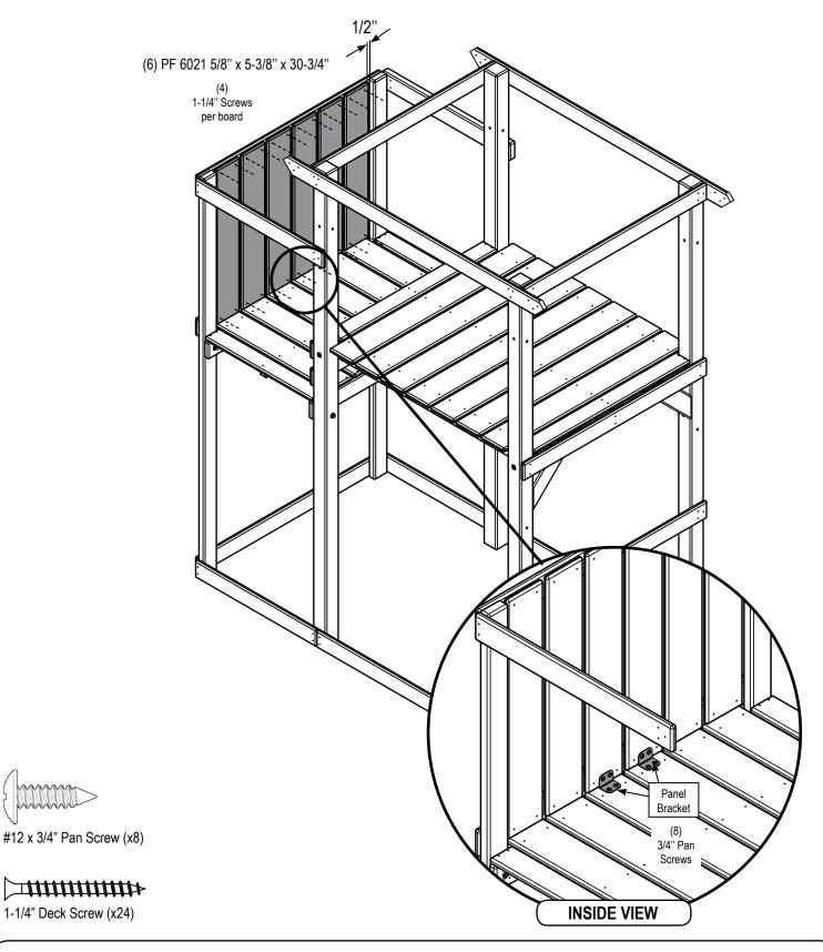
1. Install Barrier Boards as shown.
