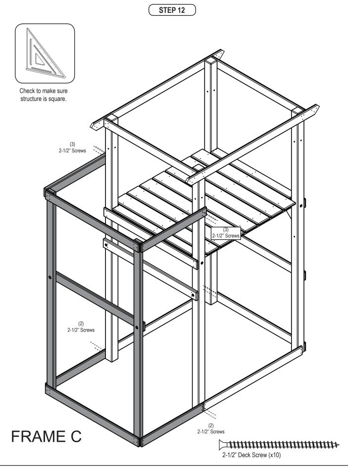
1. Attach Frame C to Tower as shown.
