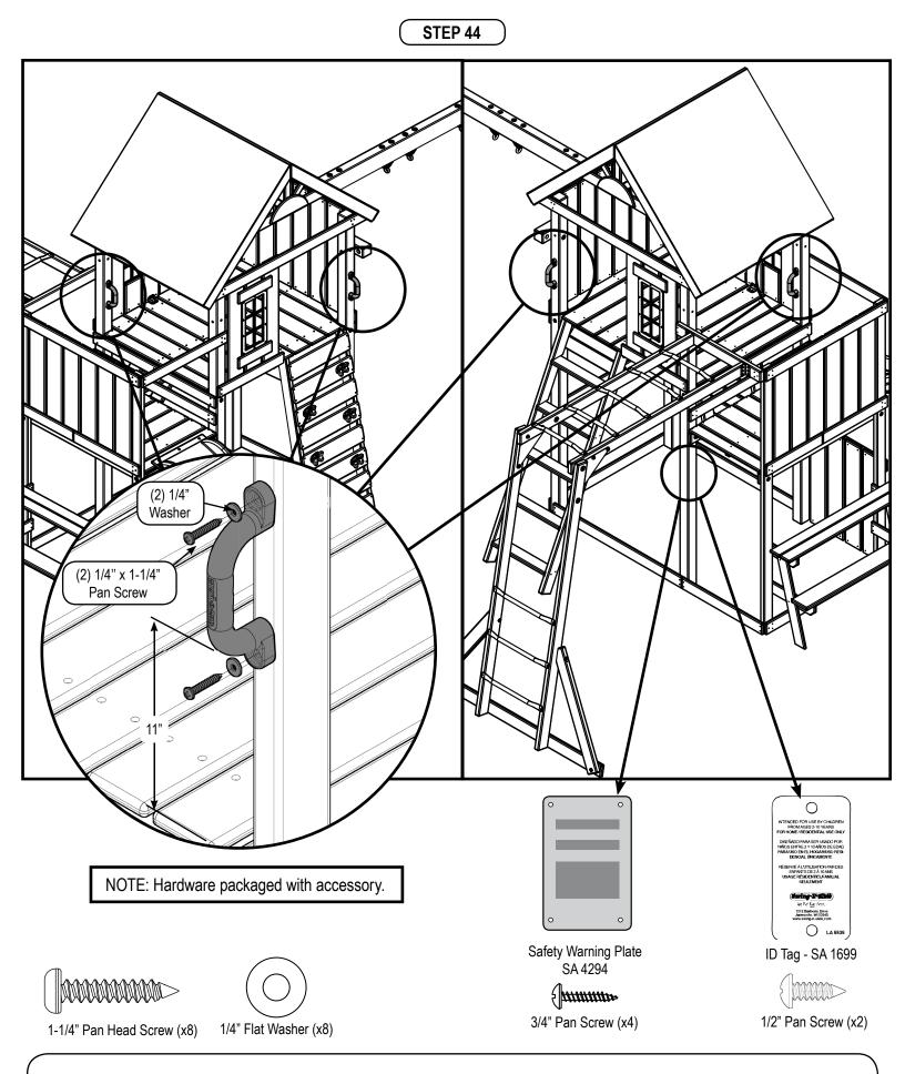
1. Attach Safety Handles, plate and I.D. Tag as shown.
