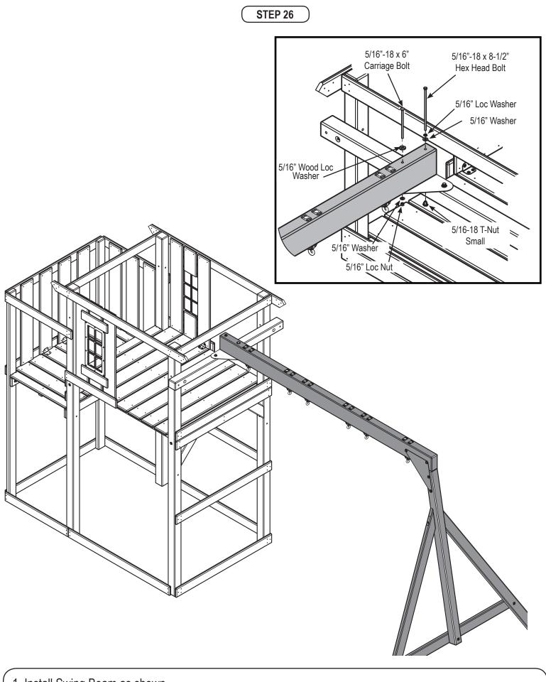
1. Install Swing Beam as shown.
