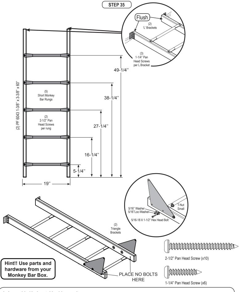
1. Assemble Horizontal Ladder as shown.
