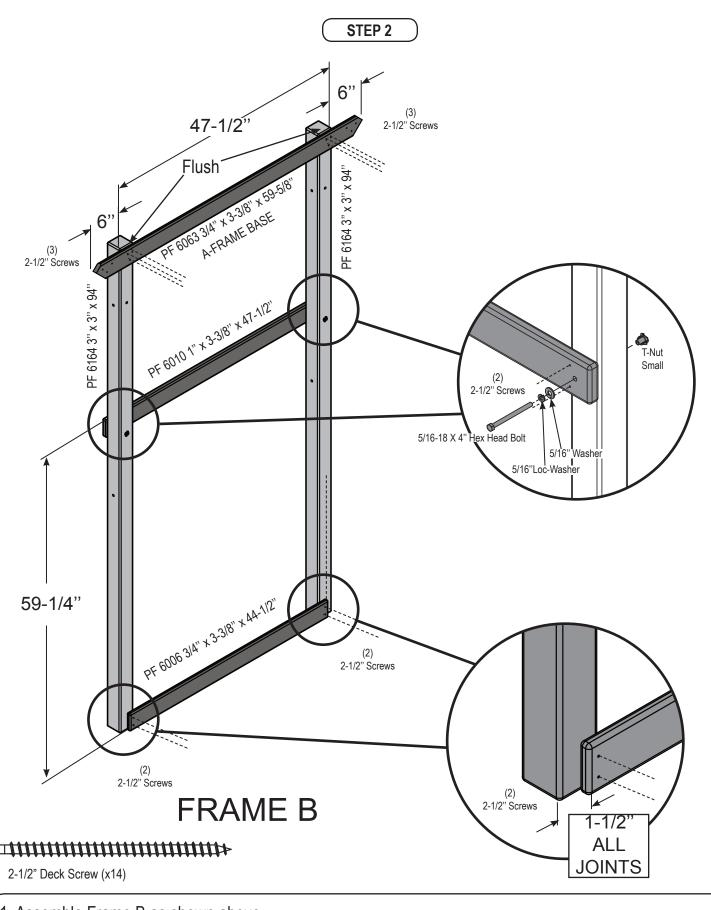
1. Assemble Frame B as shown above. **Note:** Tap each T-Nut into its pre-drilled hole until the metal tangs sink fully into the wood.
