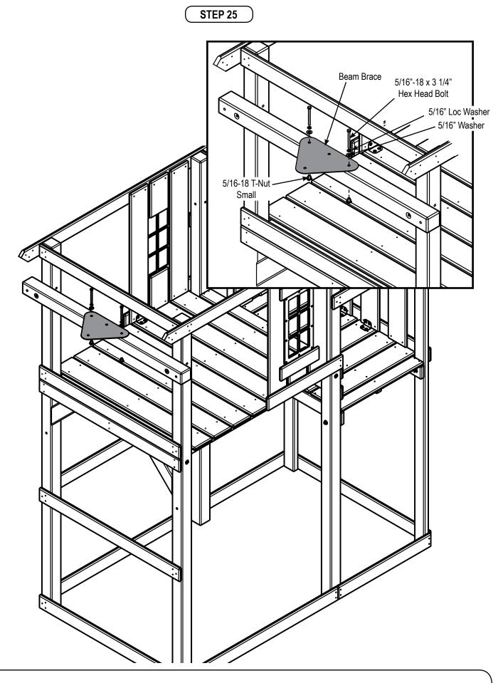
1. Install Swing Beam Brace as shown.
