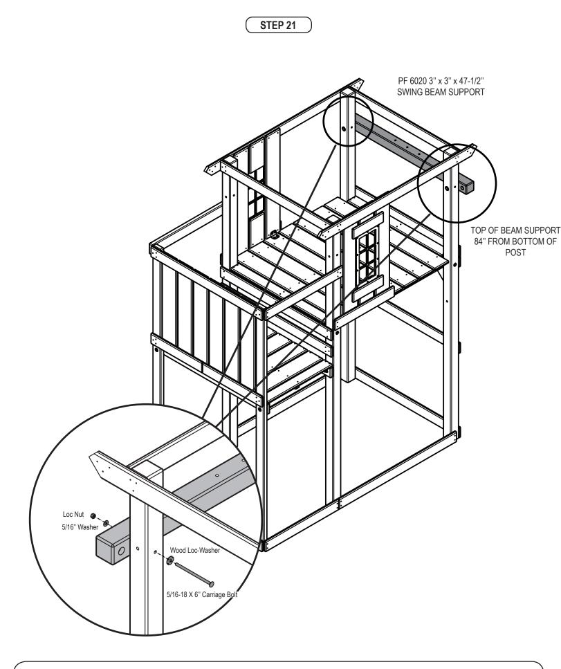
1. Install Swing beam support as shown.
