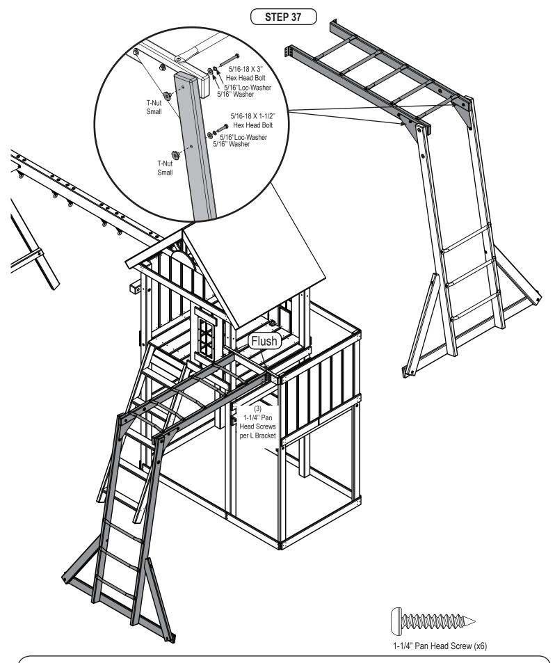
1. Assemble and attach Monkey Bar Assembly as shown.
